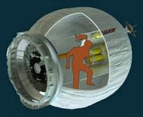
Bigelow Aerospace built a human-rated expandable habitat demonstration to be launched to the International Space Station for a two-year test.
