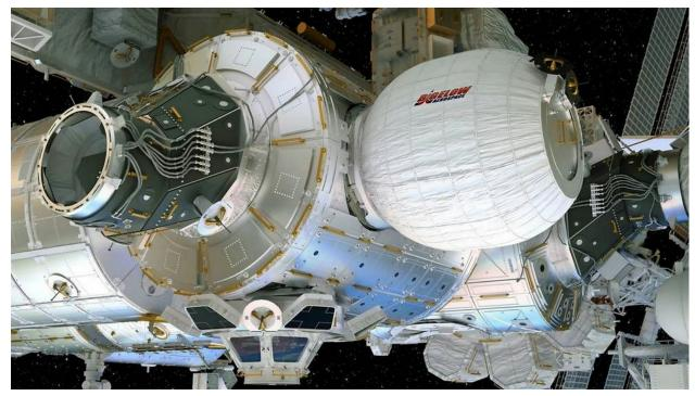
The walls consist of alternating layers of foam and a material called Nextel. These layers provide impact resistance and thermal protection as the outside temperature can vary from –200 °F (–128.9 °C) in the shade to over 250 °F (121.1 °C) in sunlight. The inner structures form an airtight bladder that contains the pressurized atmosphere. **Bigelow replaced the**Nextel cloth with Vectran and Kevlar during the reengineering process.
