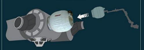
BEAM will be attached to the Tranquility Module by the robotic Canadarm2.
